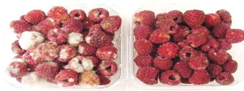
Control vs. Irradiated samples 41 days after storage at 0°C (32°F).
