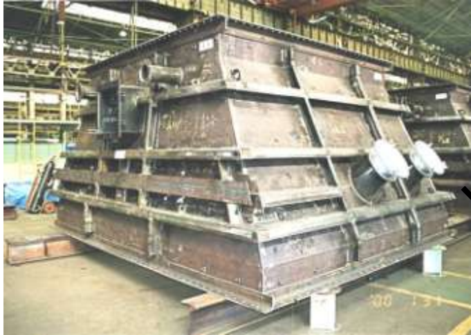
Dump Heat Exchanger (DHX) × 4
